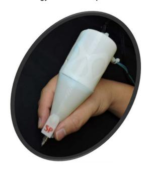
The device has potential to be adapted to different tools that include, but not limited to, pen, pencil, paint-brush, soldering iron, welding tool, tweezers, needle, pipette, knife, stylus, screw-driver, laser-pointer, and probe-based confocal laser endo-microscope.
